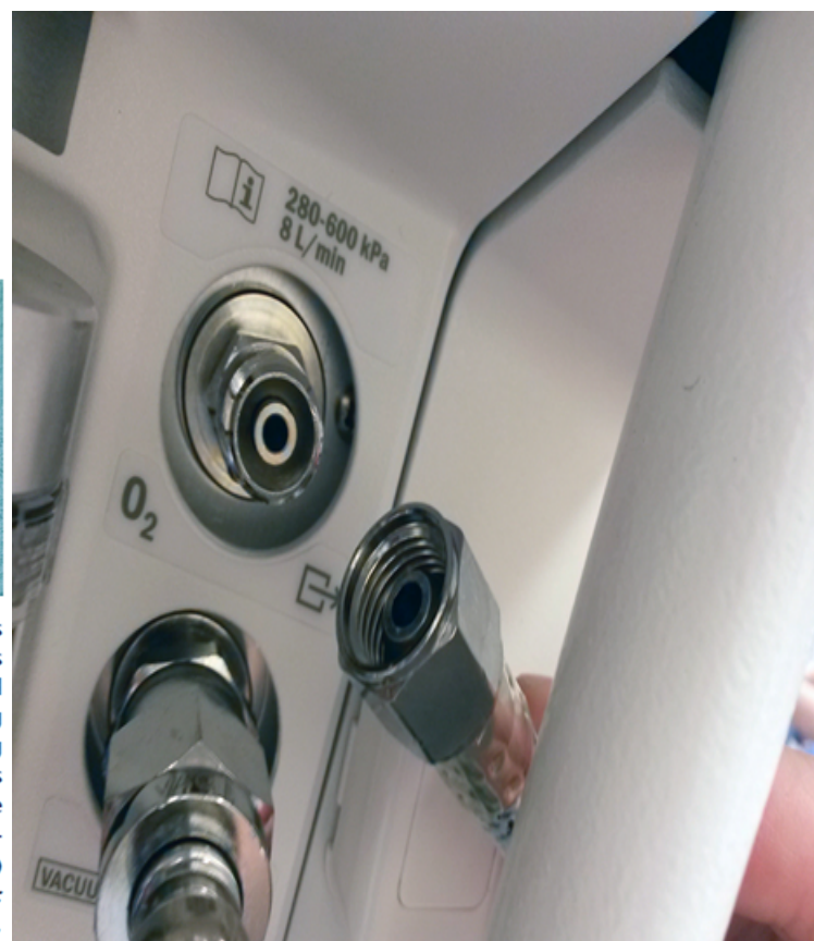
Figure 29-4. Diameter Index Safety System (DISS). DISS connectors are used for noninterchangeable, removable medical gas connections at pressures less than 200 psig. They are also used for suction and waste gas connections. Indexing is accomplished through differing diameters of the connection components, resulting in keylike fitting when matched connectors come together. The oxygen connector is additionally distinguished from the other gas connectors by a unique threaded fitting diameter and a unique thread count. A , DISS connector cross section. B , Nut and stem connectors for (left to right) vacuum, air, nitrous oxide, and oxygen. ( A , Modified from Yoder M: Gas supply systems. In Understanding modern anesthesia systems, Telford, Pa., 2009, Dräger Medical.)
