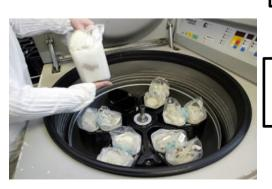
Balanced centrifuge cups are to placed diagonally in refrigerated centrifuge
