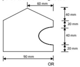
7 Calculate the moment of inertia of the section shown in figure below about xx and yy axis through the centroid.
