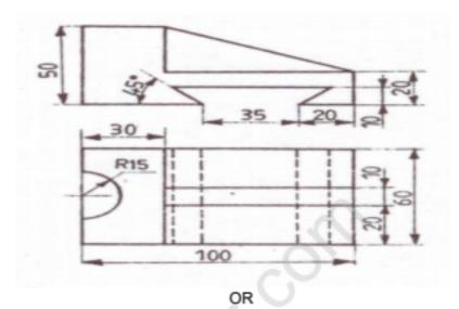
8 Draw the front view, top view and right side view of the object shown below (dimensions in mm).
