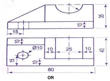
8 Draw the front view, top view and right side view of the object shown below.
