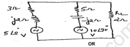
3 (a) A resistive network shown in figure, setup corresponding tie-set matrix and obtain KVL equation.
