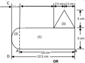
7 A thin plate of 6 mm thickness is cut and machine component is made from the plate as shown in figure given below. Assuming the density of steel as 7850 kg/m³, calculate the mass moment of inertia about z-axis as shown in figure given below.
