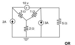
3 (a) Use mesh analysis to find  $V_x$  in the circuit shown in figure below.
