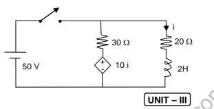
6 (a) For the circuit shown in figure below, a voltage of  $250 \sin \omega t$  is applied. Determine the power factor of the circuit.
