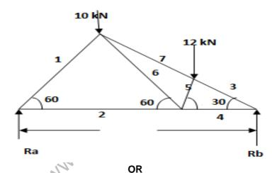
11 Find the forces in the members AB and AC of the truss show in figure below. Use method of sections.
