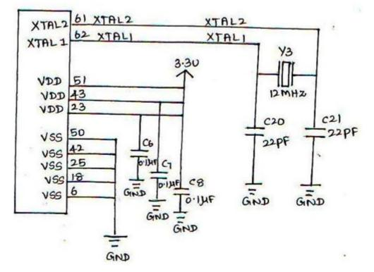
The value of capacitors C20 & C21 depends upon the frequency of crystal Y3. General circuit and its equivalent circuit is as shown below.
