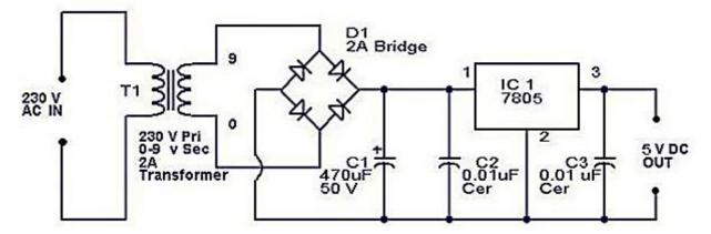
Regulator IC 7805 is used to provide fix 5V dc supply.
