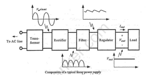
Transformer: It is used to step down 230V AC to 9V AC supply and provides isolation between power grids and circuit.
