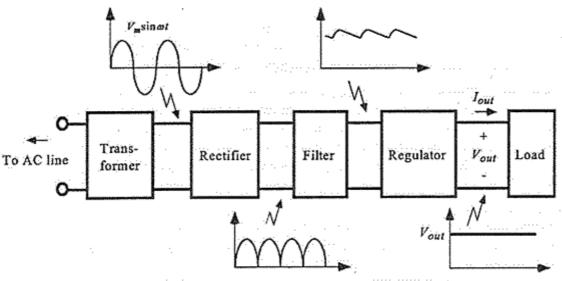
Components of a typical linear power supply
