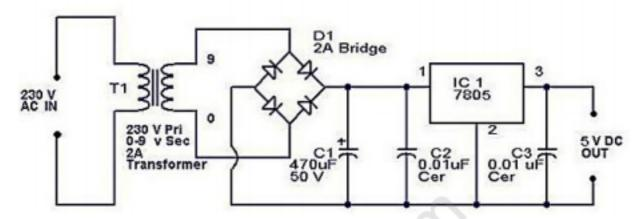
Regulator IC 7805 is used to provide fix 5V dc supply.
