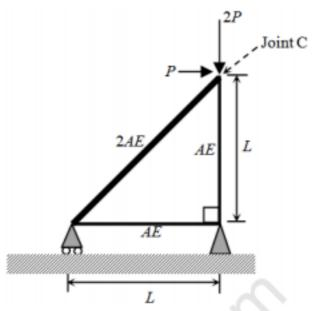
Given that  $E = 2 \times 10^{11} \text{ N/m}^2$ ,  $A = 10 \text{ mm}^2$ , L = 1 m and P = 1 kN. The horizontal displacement of Joint C (in mm, up to one decimal place) is \_\_\_\_\_
