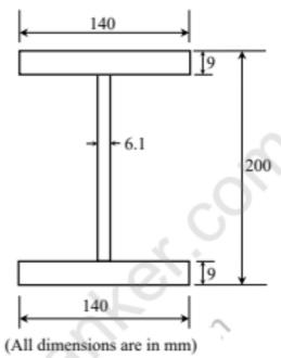
The plastic section modulus about the weaker axis (in cm3, up to one decimal place) is
