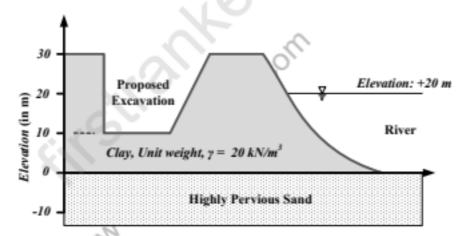
The water level in the adjacent river is at an elevation of +20.0 m. Unit weight of water is 10 kN/m<sup>3</sup>. The factor of safety (up to two decimal places) against sand boiling for the proposed excavation is \_\_\_\_\_
