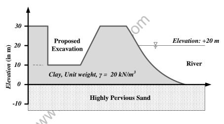
The water level in the adjacent river is at an elevation of +20.0 m. Unit weight of water is 10 kN/m<sup>3</sup>. The factor of safety (up to two decimal places) against sand boiling for the proposed excavation is \_\_\_\_\_
