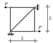
For the loads shown on the truss, the statement that correctly represents the nature of forces in the members of the truss is:
