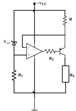
The load current  $I_0$  through  $R_L$  is
