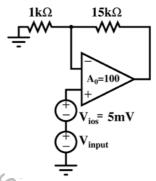
The output voltage (in millivolts) is
