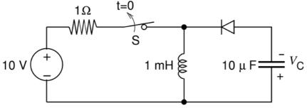
The steady state magnitude of the capacitor voltage  $V_{\mathbb{C}}$  (in volts) is \_\_\_\_
