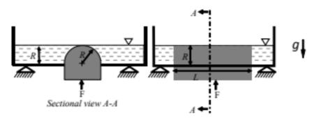
The force F required to hold the plug in its position is
