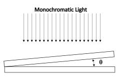
If the wavelength of light used to get a fringe spacing of 1 mm is 450 nm, the wavelength of light (in nm) to get a fringe spacing of 1.5 mm is
