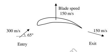
The magnitude of absolute velocity at entry is 300 m/s at an angle of  $65^{\circ}$  to the axial direction, while the magnitude of the absolute velocity at exit is 150 m/s. The exit velocity vector has a component in the downward direction. Given that the axial (horizontal) velocity is the same at entry and exit, the specific work (in kJ/kg) is\_\_\_\_\_
