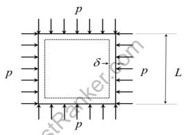
The deformed shape is a square of dimension  $L - 2 \delta$ . If L = 2 m and  $\delta = 0.001 \text{ m}$ , the Poisson's ratio of the plate material is \_\_\_\_\_
