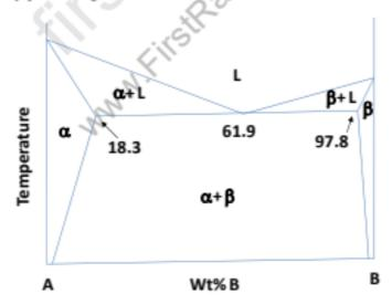
Upon complete solidification of a binary alloy system A-B, the fraction of pro-eutectic αphase present is 0.50. The alloy composition in terms of wt%. B is
