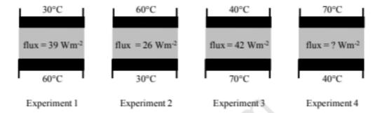
What is the steady state heat flux (in W m<sup>-2</sup>) with the top plate at 70°C and the bottom plate at 40°C?
