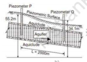
The heads indicated by two piezometers P and Q are 55.2 m and 34.1 m, respectively. The aquifer has a hydraulic conductivity of 80 m/ day and its effective porosity is 0.If the distance between the piezometers is 2500 m, the time taken by the water to travel through the aquifer from piezometer location P to Q (in days, round off to 1 decimal place) is \_\_\_\_\_.
