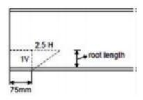
Effective area in bearing = [75 + 2.5 (flange thickness + root radius)] × 8
