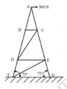
The momentum about the point A must be zero, because there is no deformation of any truss. Hence,  $F_{CD}=0$  [ $F_{CD}$  is not passing through the point A]
