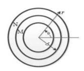
Internal pressure causes the stress in radial as well as circumferential direction.
