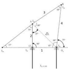
$$\begin{split} I_{24}I_{12}\omega_2 &= I_{24}I_{41}\omega_4 \\ I_{24}I_{12} &= L\tan 75^o \ (from \ \Delta \ I_{12}I_{23}I_{24}) \\ I_{24}I_{41} &= L + L\tan 75^o \\ \therefore \frac{\omega_4}{\omega_2} &= \frac{I_{24}I_{12}}{I_{24}I_{41}} = \frac{L\tan 75^o}{L + L\tan 75^o} = 0.788 \end{split}$$
