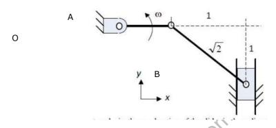
Velocity of point A,  $V_A = r \times \omega$
