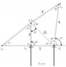
$$I_{24}I_{12}\omega_2 = I_{24}I_{41}\omega_4$$
