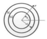
Internal pressure causes the stress in radial as well as circumferential direction.
