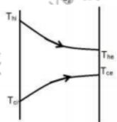
$$\begin{split} \Delta T_i &= T_{h_i} - T_{c_i} = 100 - 15 = 85^{\circ}\text{C} \\ \Delta T_e &= T_{h_e} - T_{c_e} = 82 - 45 = 37^{\circ}\text{C} \\ LMTD &= \frac{\Delta T_i - \Delta T_e}{\ln \frac{\Delta T_i}{\Delta T_e}} = \frac{85 - 37}{\ln \frac{85}{37}} = 57.71^{\circ}\text{C} \end{split}$$
