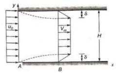
The ratio  $\frac{p_A-p_B}{\frac{1}{2}\rho u_0^2}$  (where  $p_A$  and  $p_B$  are the pressures at section A and B, respectively,
