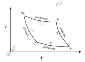
From the above Carnot cycle undergone by an ideal gas, identify the processes in which the change in internal energy is **NON-ZERO**.
