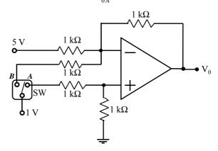
Q.13 In the bistable circuit shown, the ideal opamp has saturation levels of  $\pm 5$  V. The value of  $R_1$  (in  $k\Omega$ ) that gives a hysteresis width of 500 mV is \_\_\_\_\_.
