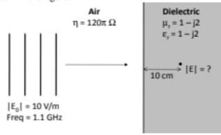
The magnitude of the transmitted electric field component (in V/m) after it has travelled a distance of 10 cm inside the dielectric region is \_\_\_\_\_\_.
