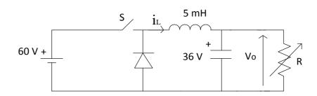
For the switching converter shown in the following figure, assume steady-state operation. Also Q.32 assume that the components are ideal, the inductor current is always positive and continuous and switching period is  $T_s$ . If the voltage  $V_L$  is as shown, the duty cycle of the switch S is \_
