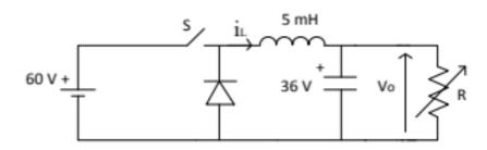
Q.32 For the switching converter shown in the following figure, assume steady-state operation. Also assume that the components are ideal, the inductor current is always positive and continuous and switching period is T<sub>s</sub>. If the voltage V<sub>L</sub> is as shown, the duty cycle of the switch S is \_\_\_\_\_.
