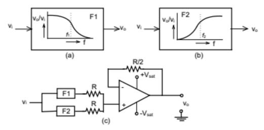
The cut-off frequencies of F1 and F2 are  $f_1$  and  $f_2$  respectively. If  $f_1 < f_2$ , the resultant circuit exhibits the characteristic of a
