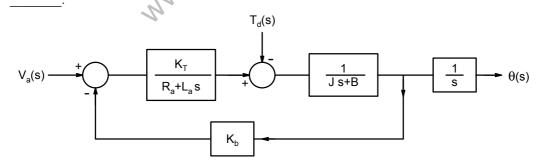
Q.47 For the system shown in the figure, s = -2.75 lies on the root locus if K is \_\_\_\_\_
