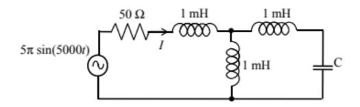
Q.31 The ABCD parameters of the following 2-port network are
