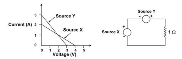
Q.31 Consider the circuits shown in the figure. The magnitude of the ratio of the currents, i.e.,  $|I_1/I_2|$ , is \_\_\_\_\_\_.
