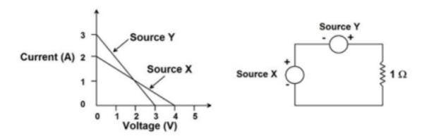
Q.31 Consider the circuits shown in the figure. The magnitude of the ratio of the currents, i.e.,  $|I_1/I_2|$ , is
