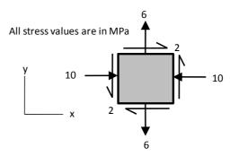
The magnitude of the maximum shear stress in MPa and its direction with the *x*-axis in degrees at the same point respectively are
