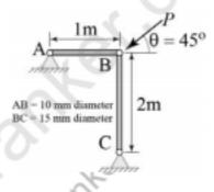
Q.21 The plane frame shown is analyzed by neglecting axial and shear deformations. The horizontal displacement of joint B is
