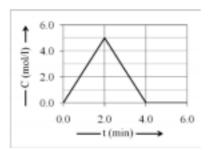
In the above figure, C is the exit tracer concentration. The corresponding E or  $E_{\theta}$  (normalized E) curve is correctly represented by which of the following choices? Here,  $\theta$  is dimensionless time.
