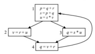
The variables which are live both at the statement in basic block 2 and at the statement in basic block 3 of the above control flow graph are
