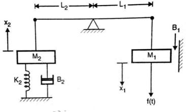
Q.3 (a) Determine the position, velocity & acceleration error constants and steady state error 03 of the system given below.
