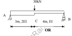
Using Castigliano's 1st theorem, calculate the deflection at point C for the beam shown in 07 (c) Figure – 1.
