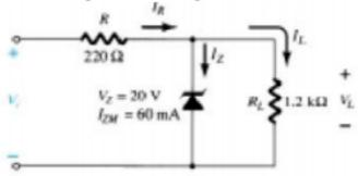
B) Determine vo for the circuit shown in fig
