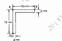
(b) The bending moment acting on the curved beam with a rectangular cross-section is M=8 KN-m. Calculate the bending stress at point B.
