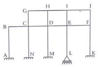
b) A braced cantilever is loaded as shown in figure. All the members are of same cross sectional area. Find the force in BE.
