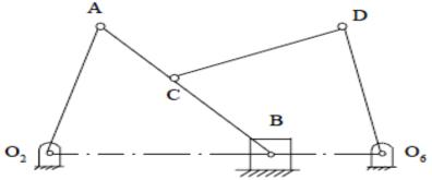
(h) Design a four bar linkage in which two successive clockwise angular displacements of 20° and 30° of the crank produce respectively, two successive angular displacements 10° and 15° of the follower.
