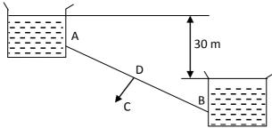
In the middle of the pipeline there is a tap through which water can be supplied to a third reservoir C. Determine the rate of flow to the reservoir B when no water is discharged to the reservoir C and the quantity of water discharged to the reservoir C is 150 lps. Neglect all losses except friction and take 4f = 0.006.
