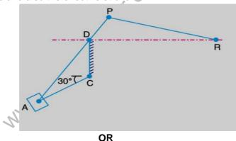
3 Give a neat sketch of the Modified Scott-Russel mechanism and Grasshopper mechanism.
