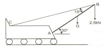
2 Determine the axial forces in the members of plane frame as shown in the below figure.
