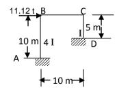
5. Determine the elements of the stiffness matrix for the portal frame with reference to the coordinates as shown in figure.
