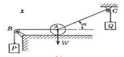
2 Determine the forces in all the members of the frame shown in below figure. Indicate the nature of forces also (Tension as +ve and Compression as -ve).
