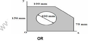
7 Calculate the moment of inertia of shaded area shown in the following figure below, with respect to the centroidal axes parallel to x axes and all the units are in mm.
