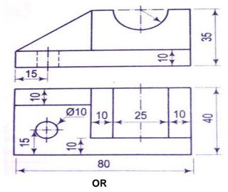
Draw the front view, top view and left side view of the block shown in figure below.(All dimensions are in mm)
