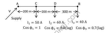
The magnitude of load currents, p.fs and distances are indicated in the figure. The resistance and reactance of each wire are 0.2 ohm and 0.3 ohms per km respectively. It is required to maintain voltage at point B as 230 V, find:
