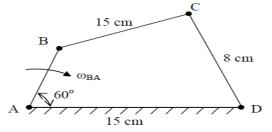
(b) In a crank and slotted lever mechanism shown below, crank rotates of 300 rpm in a counter clockwise direction. Find: (i) Angular velocity of connecting rod. (ii) Velocity of slider.
