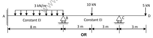
Analyze the continuous beam shown in figure below, using moment distribution method. Draw shear force and bending moment diagram for the continuous beam.
