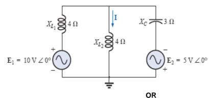
9 For the following figure. Find the Thevenin equivalent circuit, load current and power consumed by load.
