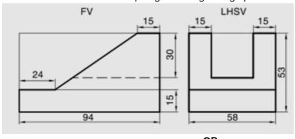
Draw the orthographic views of the object given in figure below.
