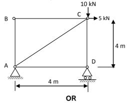
7 Compute the vertical deflection and horizontal displacement of joint D of the truss shown in figure below. The cross sectional areas of the members in square centimeters are shown in parentheses.
